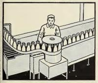
Last of all, another clever machine fits on an air-tight paper cap. No dirt can get into the bottles. The bottles sparkle in the bottling plant because they have been washed so well. Each one is washed nine times before it is ready for the milk.
